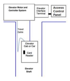
Once you start restricting many floors to different card privileges (known as destination control) you may need lots of outputs, we can add up to 64 outputs per controller using extension boards.
