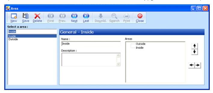
Then, for each reader located between two areas open the **Controller>Reader>Door Control** screen and fill the area path (eg. the entrance reader should have **From 'Outside' to 'Inside'**, the exit reader should have **From 'Inside' to 'Outside'**). For the other readers, fill the area path with the same area (eg. if the reader is inside, it should be set **From 'Inside' to 'Inside'**).
