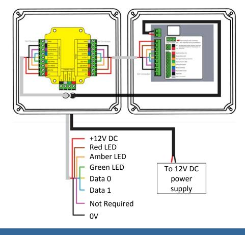
You will see that the interface is mounted upside down in the housing. This is to position the internal aerial away from other reader components and is intentional.
