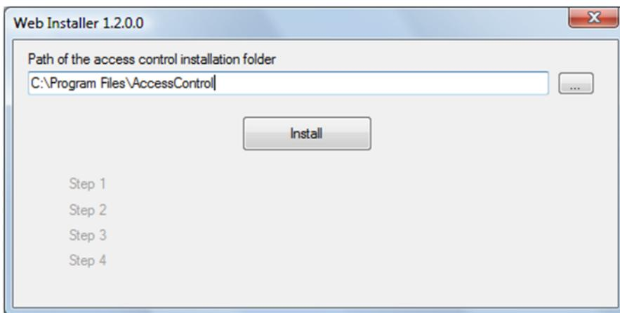
After selecting the path where is your Access control software is located (typically C:\Program Files\GuardPointPro), Click **Install** button.
