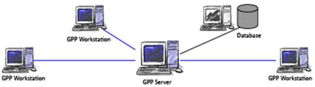
The GuardPoint Pro server redundancy principle is to provide the server function in case of failure of the mair server.
