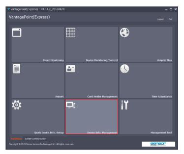
At the Device Info. Management window: Highlight the controllers you wish to batch upload to [1] Select the System Functions tab [2] Click the Device Information radio button [3] Ensure from the Controller List all controllers to be batch uploaded to have a tick in their check box [4] Click the Upload button [5]
