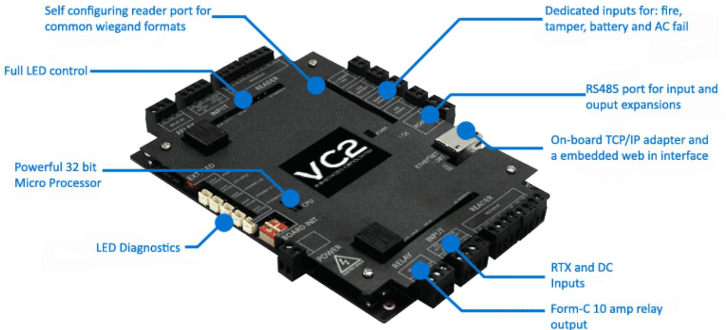
**The Vantage Controller is a powerful Ethernet ready four reader controller that provides advanced and easy solutions for any size of application. This controller works with our Vantage Point Software.**
