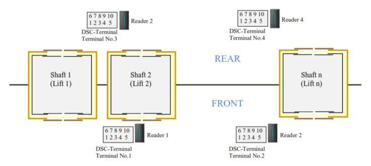
One controller is installed at each floor, which can manage the readers of the floor, and all the controllers are connected to their RS485 Port 2. The RS485 bus is connected to the Thyssen LCS via a RS485/RS232 convertor.
